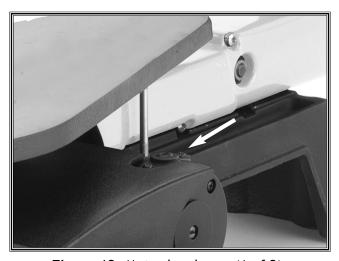
Figure 13. Motor brush cap (1 of 2).
